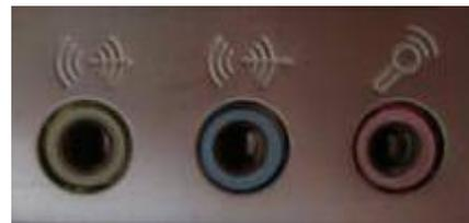
input for devices such as guitar preamps, hardware drum machines, or any component that has an audio output. And the green is your speaker or headphone output.
