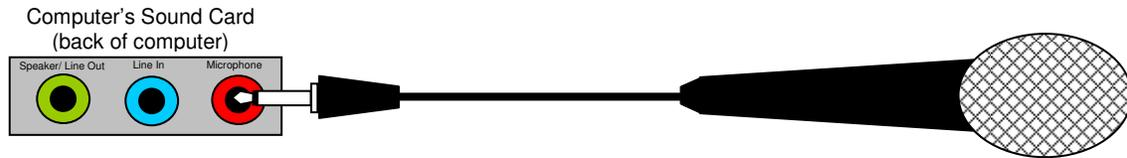
Connecting a Microphone with a 1.5mm plug to the soundcard
